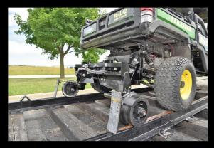
Our optional Composite Rail Wheels have and hardened steel tread with aluminium inner separated by special dialectic neoprene that cuts down on rail head noise up to 95%. The Rail Wheels are naturally insulated.
