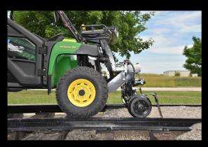
Our Flexiride® Rail Gear has 4 wheel independent suspension that self-compensates for uneven track conditions. The basic system is provided with a self-contained hydraulic power unit with emergency hand pump, front and rear rail sweeps, outside push button controls and replacement tires.
